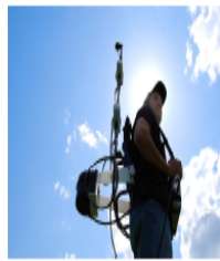
Walking Gradiometer with VLF-EM and GPS
